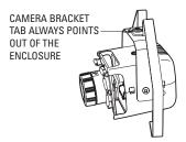
**Wall Mounting** – The camera bracket tab points out of the enclosure and the top of the camera points up towards the tab.
